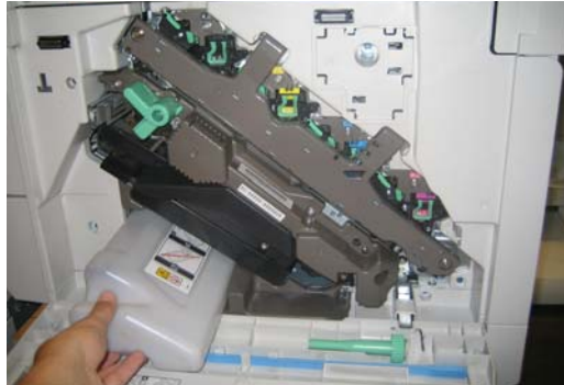
Imaging unit revealed while the waste toner bottle is replaced
