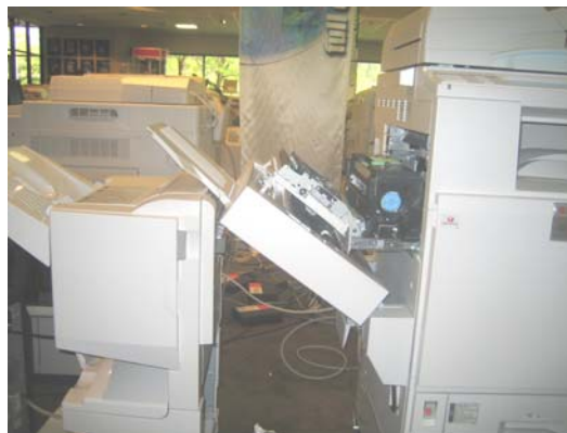
Finisher being rolled away to gain access to the duplex unit
